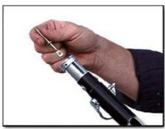
Insert 1/4" x 3" accoustical lag screw into top slot.
