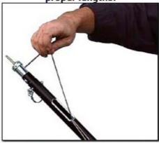
Insert wire into side of slot, through the hold in the lag screw. Then bend the wire end down.
