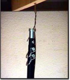
Rotate the tool again to twist the wire. LagMaster may be turned by hand or by using a 1/2" variable speed drill. Caution: if using drill, do not grip pole tightly with hand, but allow it to turn loosely.
