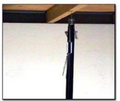
Raise tool against beam or joist, rotate LagMaster until the Lag is at least 1" into the wood.
