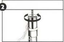
Secure a #1 1/2 "S" hook to an acoustical eye lag and to the proper size chain for your job. Insert it into the LagMaster Plus. Secure the chain in the magazine so it does not whip when rotating the pole. Now rotate the eye lag linsert it into the LagMaster Plus. Screw until it is seated.
