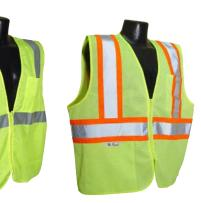
**Garment is made from 100% Polyester Treated** to be Self-Extinguishing as defined by ASTM D6413 (<2.0 Second Flameout / <6.0" Char Length). This garment should never be used where an arc flash or flash fire hazard is present. This garment is not flame resistant as defined by ANSI/ISEA 107-2015 Section 10.5 Self-extinguishing properties diminish with washing.
