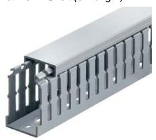
**NARROW SLOT-** Smaller, tighter number of fingers for more concise harnessing. Finger design restricts wire from slipping along the edge, creates 2 or 3 levels of wire service.
